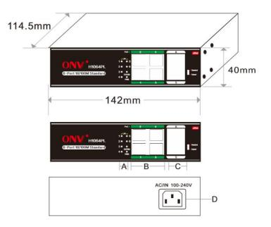
A. Working indicator B. 4x10/100M PoE ports C.2x10/100M Uplink Rj45 ports D. Power input port AC100-240V,50/60Hz
