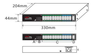
A.Multi-functional switch B.Working LED indicator
