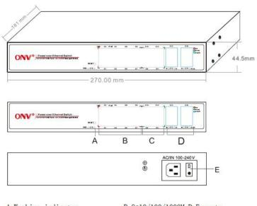
A. Working indicator B. 8\*10/100/1000M PoE ports C. 4\*10/100/1000M RJ45 ports D. 4\*1/10G SFP+ ports
