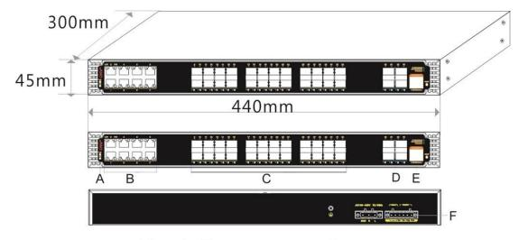
A.Working indicator C. 24\*Gigabit SFPPorts E.Console port B. 8\* PoE Ports D.4\*1/10G SFP+ Ports F.AC/DC dual input port
